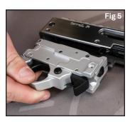
**DO NOT** spray any oil onto the hammer/sear engagement area. Be sure to remove any excess over spray with a cotton swab.
