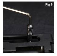
DO NOT disassemble the bolt any further. The inside of the receiver should be cleaned and minimally lubricated on a regular basis using any quality gun oil.
